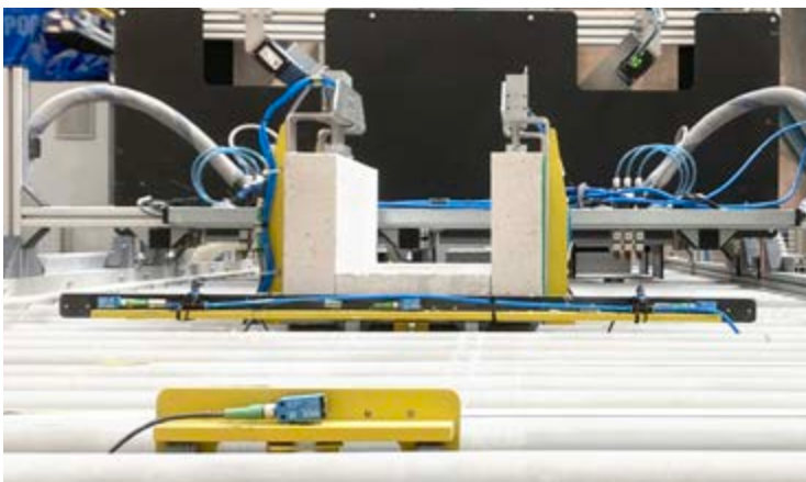
Here the three concrete parts are glued together to form a U-profile.
